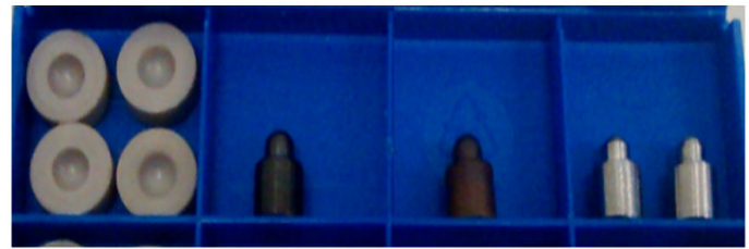
Figure 2. Bearings in PEEK left; followed by pivot in titanium with DLC, pivot in PEEK with DLC and pivot in pure titanium.
